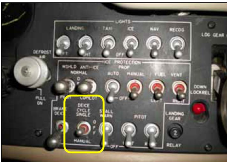
Figure 4: Raytheon B200 ice protection panel (typical) – wing and horizontal stabilizer de-ice control switch highlighted
