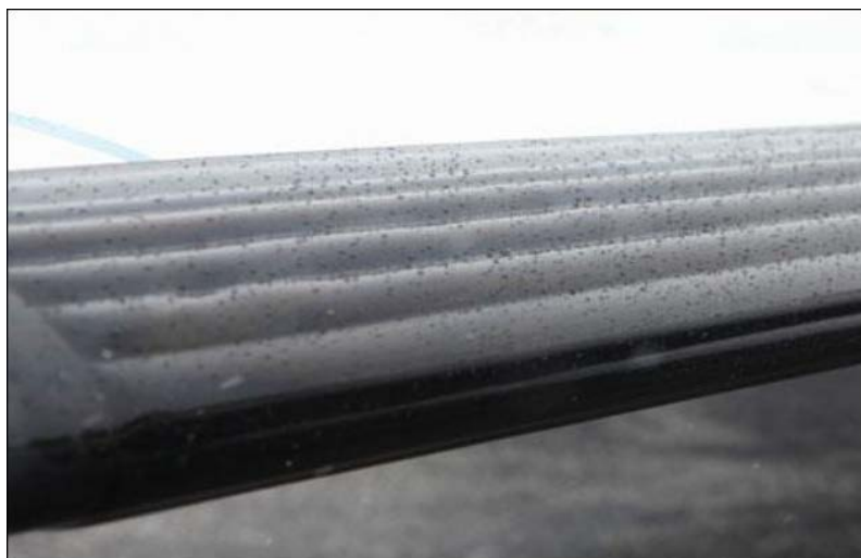
Figure 3: Inflated Raytheon B200 wing leading edge de-ice boot
